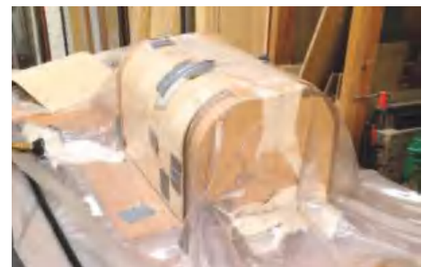
Doors being formed in vacuum bag
